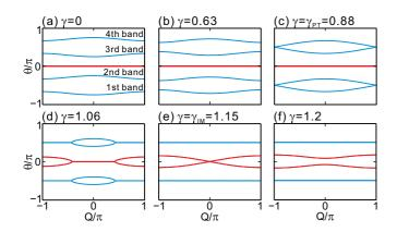
FIG. 2. (a)–(f) Band structures for  $\gamma = 0, 0.63, 0.88, 1.06, 1.15,$  and 1.2, respectively. The blue and red lines represent the real and imaginary parts of the propagation constant, respectively.
