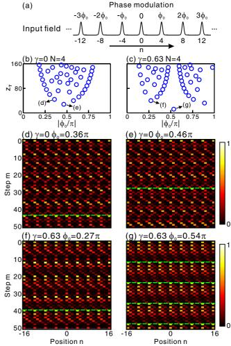
FIG. 4. (a) Schematic of the linear phase modulation imposed on the input field. (b), (c) Talbot distance  $z_T$  versus  $|\phi_0|$  for  $\gamma = 0$ and 0.63, respectively. The incident period is N = 4. (d), (e) Talbot carpets for  $\phi_0 = 0.36\pi$  and  $\phi_0 = 0.46\pi$ , respectively.  $\gamma$  is set as 0. (f), (g) Talbot carpets for  $\phi_0 = 0.27\pi$  and  $\phi_0 = 0.54\pi$ , respectively.  $\gamma$  is chosen as 0.63.
