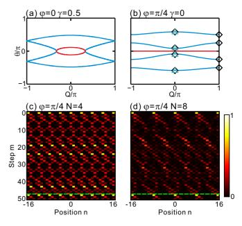
FIG. 8. (a) Band structures for  $\varphi = 0$  and  $\gamma = 0.5$ . (b) Band structure for  $\varphi = \pi/4$  and  $\gamma = 0$ . The modes contained in the field evolution for N = 4 and 8 are represented as the cyan triangles and black diamonds, respectively. (c), (d) Talbot carpets for N = 4 and 8, respectively.  $\varphi$  and  $\gamma$  are chosen as  $\pi/4$  and 0, respectively.
